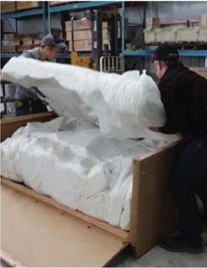
Figure 4: Lift monolithic foam straight up and over, there may be a top and sides or just one large piece.
