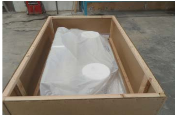
Figure 2. Crate side walls are attached to the base and the crate contents are covered with a protective layer of plastic wrap.
