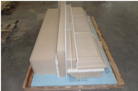
Figure 1. The bottom of the shipping crate is attached to a shipping pallet. Stones are laid on an initial layer of foam and then stacked side-by-side and atop one another with a protective sheet of Styrofoam between all stone edges and faces.
