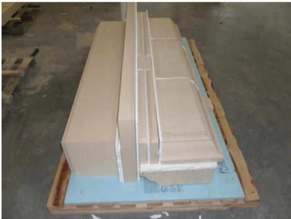
Figure 1. The bottom of the shipping crate is attached to a shipping pallet. Stones are laid on an initial layer of foam and then stacked side-by-side and atop one another with a protective sheet of Styrofoam between all stone edges and faces.
