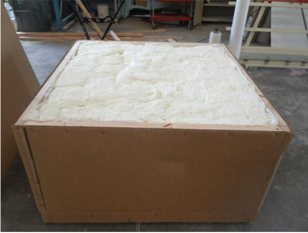
Figure 3. The crate is then shot with expanding foam to secure all parts as one in a monolithic package.
