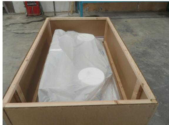
Figure 2. Crate side walls are attached to the base and the crate contents are covered with a protective layer of plastic wrap.
